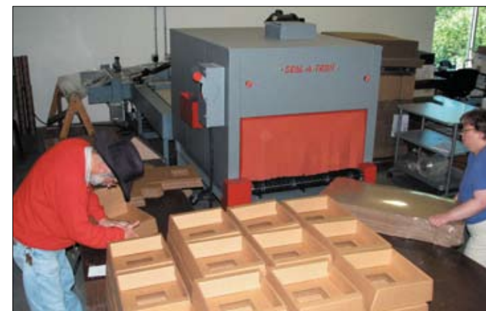
Edwards Enterprises employees John Sunday (left) and Annette Elder work the new shrink wrap machine, purchased with a gift from the William G. Gilmore Foundation. The largest of its kind in the tri-county area, the machine can package items as large as 3-by-4 feet, as well as smaller things such as books and toys.
